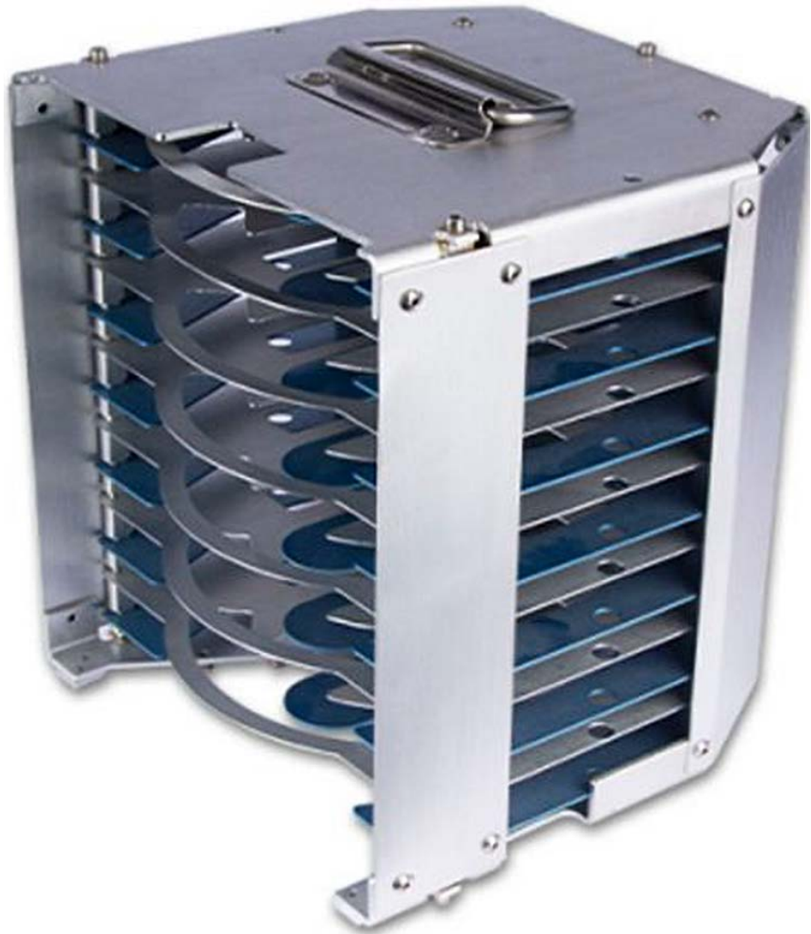
8" 7 slots of wafer cassette for BGA special use,E12 type Art. No.: DSF20E12 Size: 345×293×328 mm Material: AL 6061 DIST: 10mm Wide: 3.5mm Depth: 18.5mm
