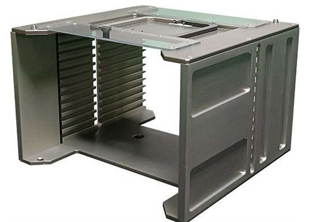
8" 13 slots of wafer cassette,A78 type Art. No.: DSF20A78 Size: 286x276x191 mm (Material): AL6061 (Slot distance): 13mm (Slot width): 7mm (Slot depth): 5.6mm
