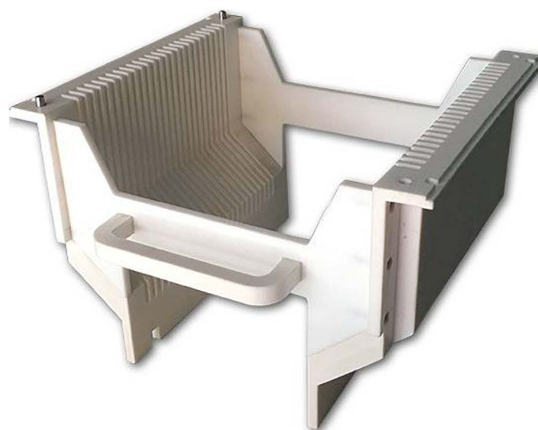
8" 25 slots of wafer cassette,R08 type Art. No.: DSF20R08 Size: 294.7x159x227.5 mm (Material): PFA (Slot distance): 6.35mm (Slot width): 3mm (Slot depth): 11.5mm
