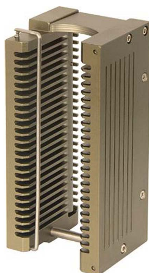
2" 25 slots of anti-skip wafer cassette,B02 type Art. No.: DSF20B02 Size: 62x62x142.6 mm (Material): AL 6061 (Slot distance): 4.76mm (Slot width): 1.6mm (Slot depth): 8mm
