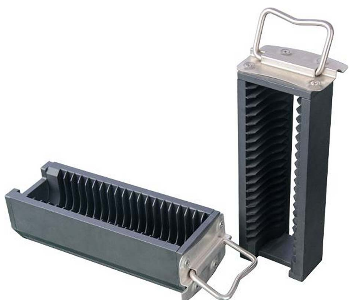
2" 25 slots of wafer cassette,A02 type Art. No.: DSF20A02 Size: 68.8x59x197mm (Material): AL 6061 (Slot distance): 7.7mm (Slot width): 6.7mm (Slot depth): 7mm
