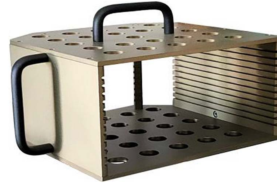
12" 12 slots of wafer cassette,I12 type Art. No.: DSF20I12 Size: 255×204.5×303 mm Material: AL 7075 DIST: 10mm Wide: 3.5mm Depth: 13.5mm
