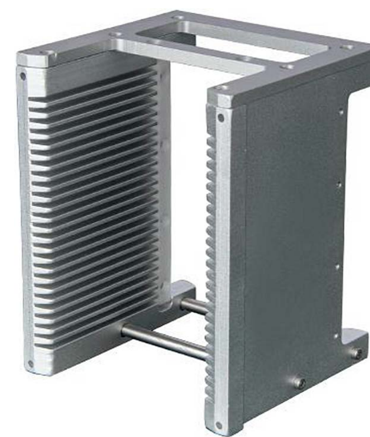
4" 25 slots of wafer cassette,A03 type Art. No.: DSF20A03 Size: 94x83x148.1 mm (Material): AL 6061 (Slot distance): 4.76mm (Slot width): 1.6mm (Slot depth): 8mm
