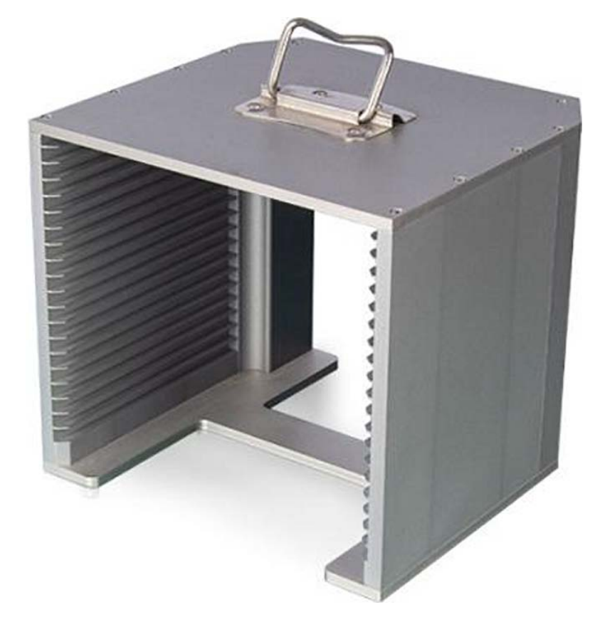
8" 20 slots of wafer cassette,E08 type Art. No.: DSF20E08 Size: 218x203x197 mm (Material): AL 6061 (Slot distance): 7.7mm (Slot width): 6.7mm (Slot depth): 7mm
